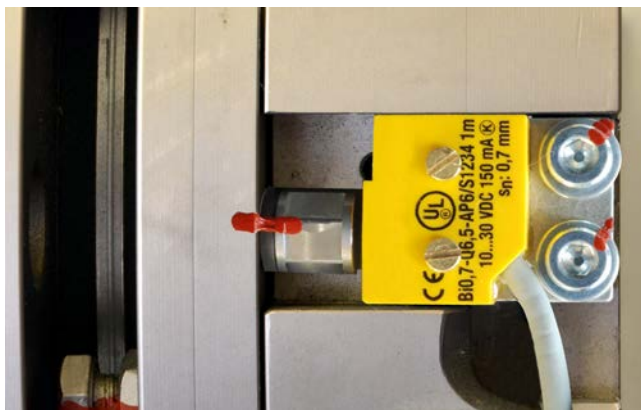
Contactless release monitoring with inductive proximity switches
